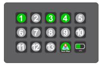
Press and hold any un-programmed station button (grey) for 3 seconds until you hear the double-beep sound. Station button will turn green, indicating programming completed.
