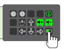
**That's all there is to it!** You have programmed MARC and can put him to work right away. Press the location button for each programmed key (in our example 1 and 3) and MARC will travel to the destination programmed for that button. Add more locations as needed and leverage the benefits of automation!
