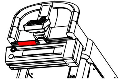
**NOTE:** If you are unable to use the info button for some reason, the serial number can also be found on the label attached to the metal battery bracket under the handle of the cart (shown in red at right).
