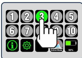
TIP: If you see the second screen, press the battery level button to return to the first screen with station buttons 1-10.
