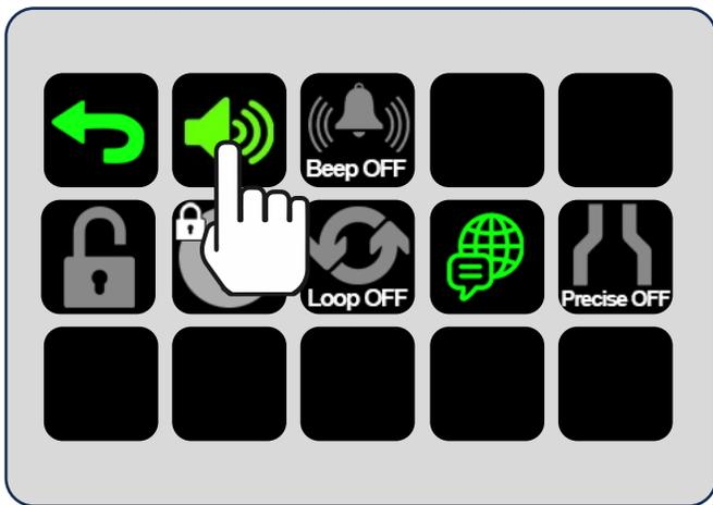
Once the Volume menu icon turns grey, you can now lock the cart and the volume adjustments will not be available to users. The volume level you set will remain until the cart is unlocked and the setting changed.
