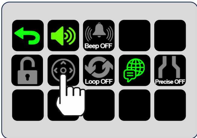
Once the Power Assist setting is set how you want it (accessible or not), you can lock the cart and the Power Assist function setting cannot be changed by users. If the setting is enabled (green) it cannot be disabled without unlocking the cart with the security code.
