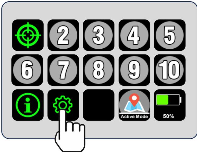
MARC carts can be locked for preventing users from changing certain settings. This includes the volume settings. If you want to ensure that the volume does not change from the desired setting, you can use the EZ-Go Navigation locking function to accomplish this. Note that some functions are automatically fully locked, and others are optionally part of the locking settings.
