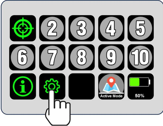
MARC carts can be locked for preventing users from changing certain settings. This includes the beep settings. If you want to ensure that the beep does not change from the desired setting, you can use the EZ-Go Navigation locking function to accomplish this. Note that some functions are automatically fully locked, and others are optionally part of the locking settings.
