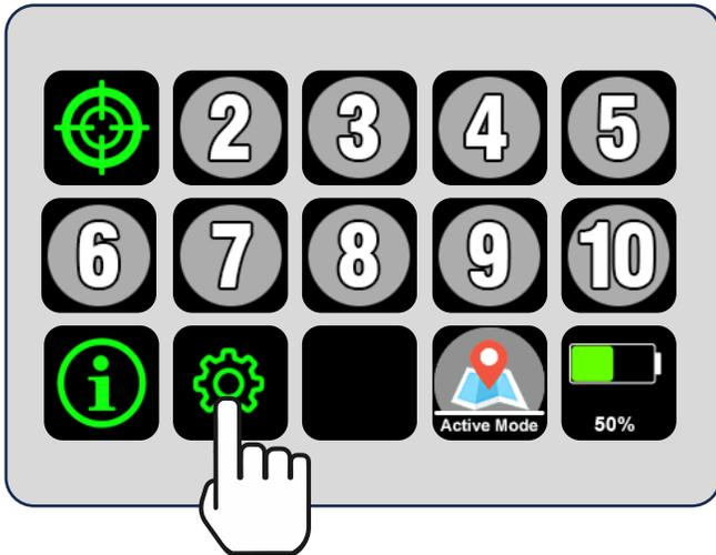
MARC carts can be locked for preventing users from changing certain settings. This includes the looping mode settings. If you want to ensure that the looping mode state does not change from the desired setting, you can use the EZ-Go Navigation locking function to accomplish this. Note that some functions are automatically fully locked, and others are optionally part of the locking settings.
