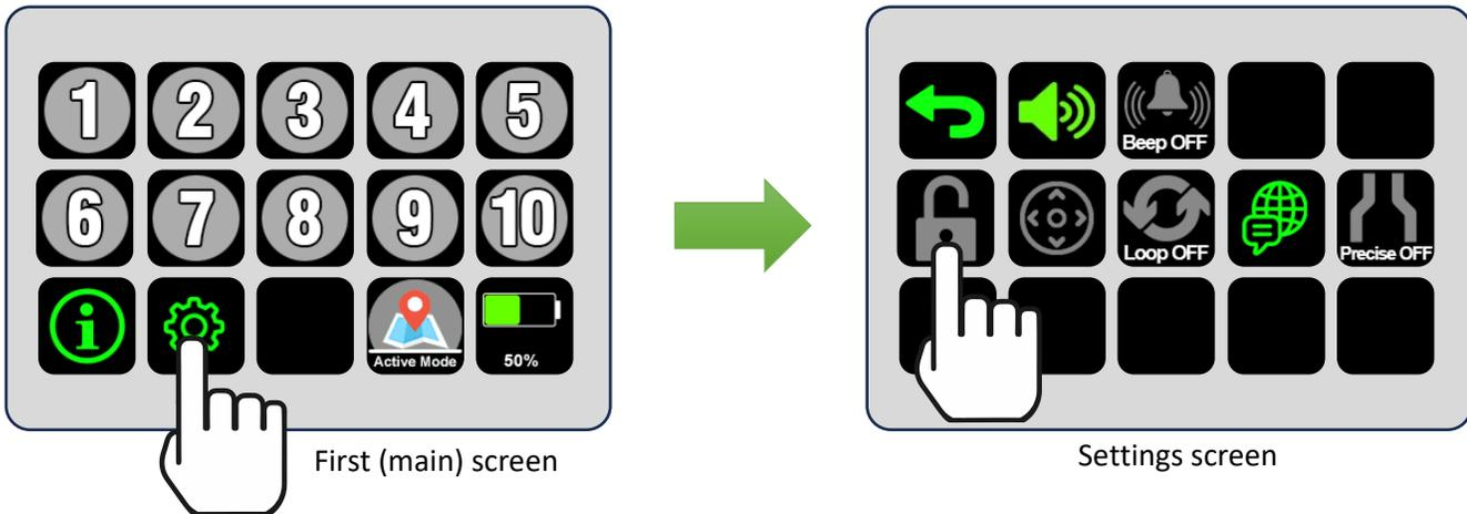
Some settings are automatically locked to prevent user changes. Others are locked in an enabled or disabled state. For example, all destination buttons are automatically locked in their current state, while the volume level submenu remains locked in either an on or off (accessible or not accessible) state – based on the status when the lock code is applied.
