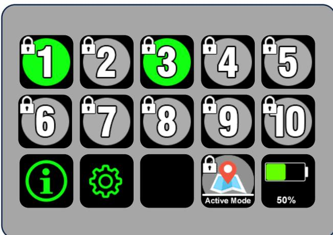
Once the cart has been locked, buttons will show padlock as indication that they cannot be changed till the cart is unlocked.
