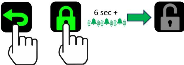
Press and hold the padlock icon for over 6 seconds till you hear the triple-beep audio cue. When you release the button, the padlock will turn grey and appear unlocked, indicating that the cart is now unlocked.
