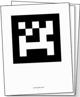
AprilTags are a form of two-dimensional barcodes designed for reliable detection and identification by computer vision systems. They consist of a black-and-white square grid with a unique pattern that encodes a specific identifier. This identifier can be decoded by a camera and associated algorithms to determine the tag's position and orientation relative to the camera's viewpoint. The simplicity and robustness of AprilTags make them ideal for various applications in robotics and automation.
