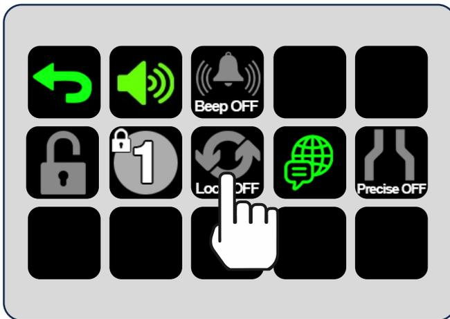
Once the Looping Mode is set how you want it (on or off), you can lock the cart and the looping mode setting will not be available to users. The cart will remain in looping mode until the cart is unlocked and the setting changed.
