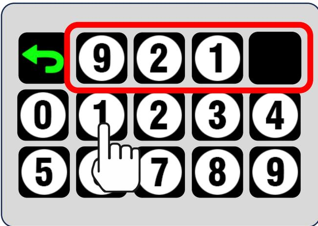
Enter the 4-digit numerical code you would like to use to lock the cart. Once the code is entered, tap the back arrow to return to the previous screen displaying the lock icon.
