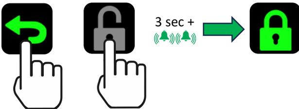
Press and hold the padlock icon for over 3 seconds till you hear the double-beep audio cue. When you release the button, the padlock will turn green and appear locked, indicating that the cart programming is now secured.
